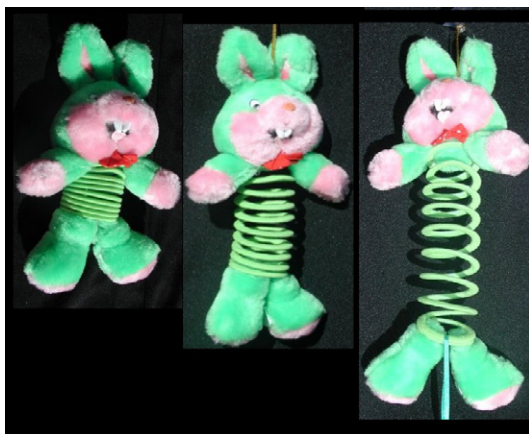
Figure 1. A spiral rabbit has an internal spring scale measuring the force acting on the feet or head. The figure shows the look of the rabbit for weightlessness ( 0g ), normal load ( 1g ) and for a motion giving 2g (e.g. as in an upward acceleration of 1g ). The resolution can be increased by holding the rabbit upside down, since the head is heavier.
