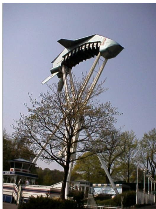
Figure 6. An amusement ride where riders sit about 13 m from the centre, but with a half-period of about 10 s (for small angles). The long period is due primarily to the counterweight, partially hidden behind the tree. Since this pendulum is rigid, rather than suspended in a chain, it is possible to complete a 360° turn, nearly stopping at the top.
